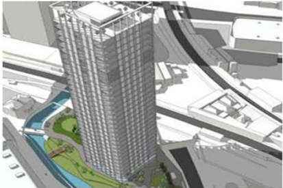
Lewisham, London High density development featuring a 35 storey tower on a constrained site with challenges that include easement corridors for Thames Water, DLR, Network Rail and the enhancement and naturalisation of the Ravensbourne River flowing through the site.
