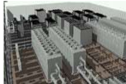
Infinity, Slough & London 2 Full structural and civil design of data space delivered across 3 phases with Uptime Institute Tier 4 certified design. Scheme involved new mezzanine floors built on screw pile technology within an existing live facility
